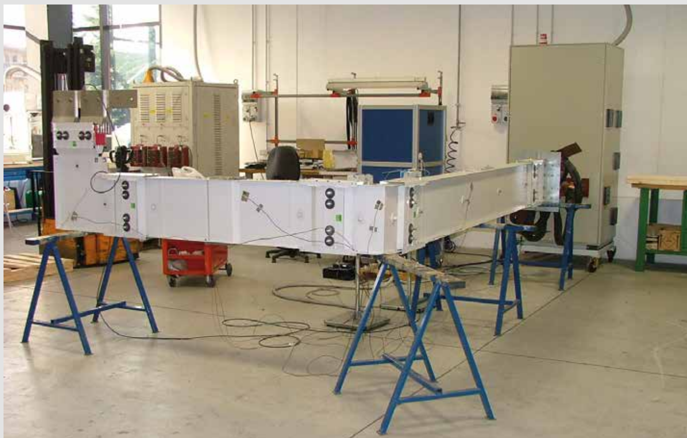
The Legrand lab during the tests for the approval certification of SCP busbar trunking systems
